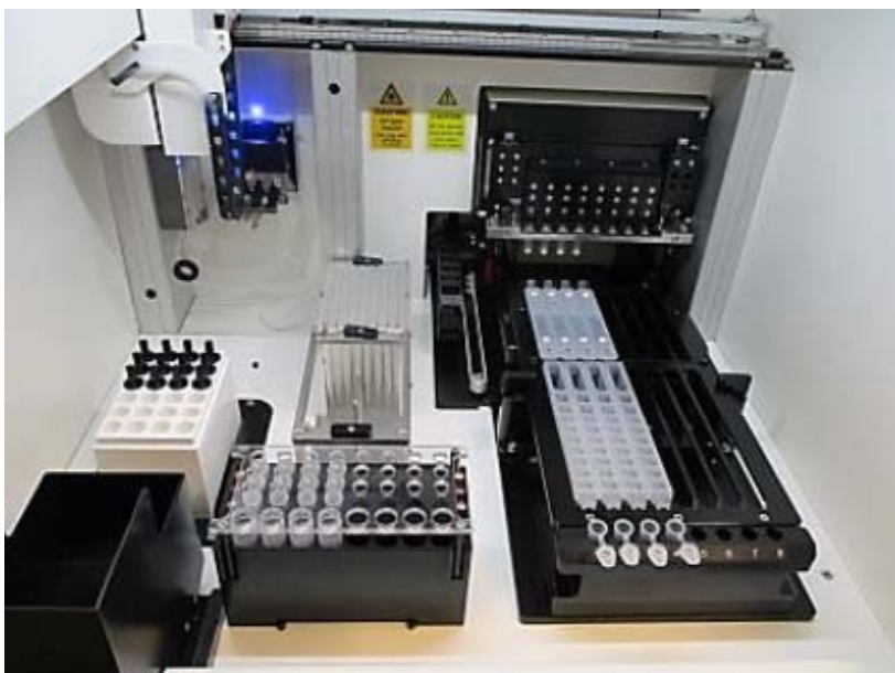
Patho-Robot loaded with consumables for enrichment and extraction of microbial DNA from 5 ml samples.
